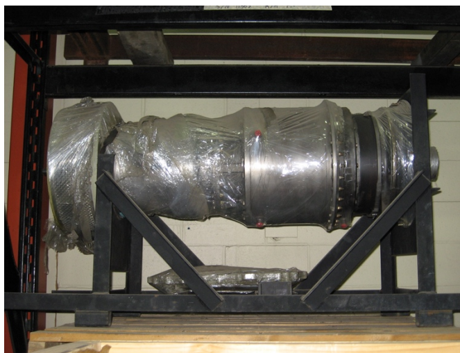
Overhauled, 0 Hour Solar T1401 Gas Turbine
