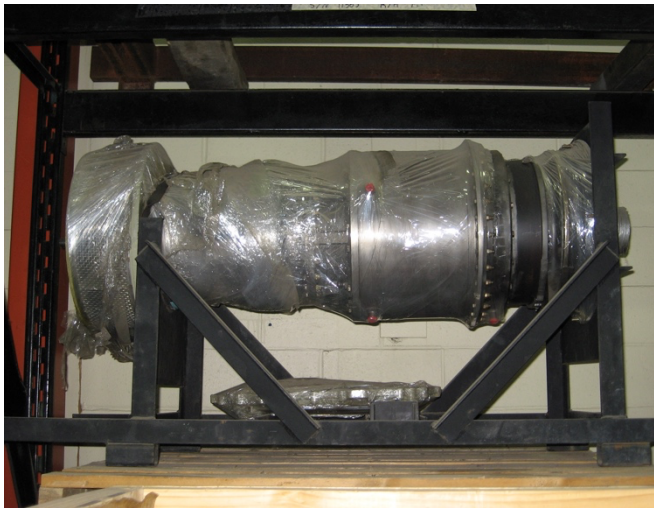
Overhauled, 0 Hour Solar T1401 Gas Turbine
